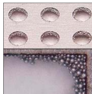
Figure 1 – Solder paste build up
